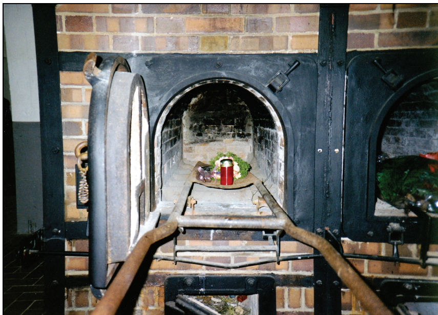
Document 44: Crematorium of Mauthausen. Topf coke-fired double-muffle oven, Auschwitz type. Loading system of oven: fixation shaft, mobile roller system and corpse stretcher. Viewed from above. © Carlo Mattogno.
