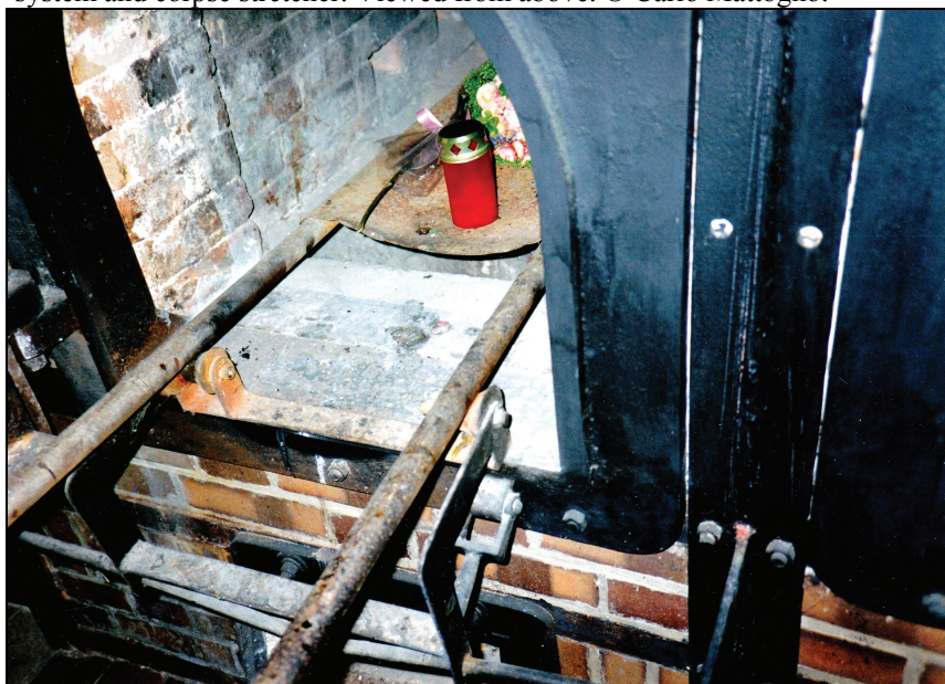
Document 45: Crematorium of Mauthausen. Topf coke-fired double-muffle oven Auschwitz type. Loading system of oven: fixation shaft, mobile roller device supporting the bars of the corpse stretcher. © Carlo Mattogno.
